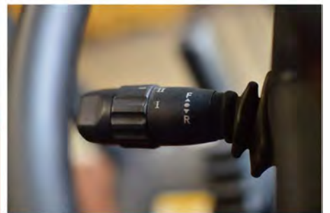
Ergonomic instrument panel: integrated handle switch, ratchet type hand brake and integrated electro-hydraulic reversing handle
