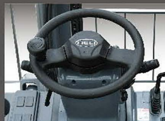
Independent steering system supplies oil for steering on demand and reduces truck energy consumption.
